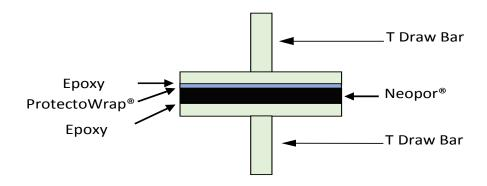
Figure 1. Sample set-up for Adhesion Testing
